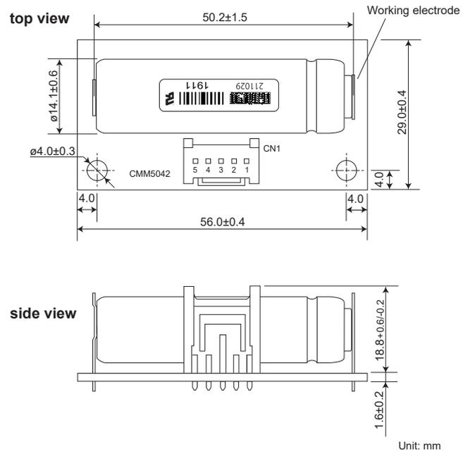
\*1 If the water in the reservoir should freeze very rapidly (typically occurs only under artificially created conditions), irreversible change of sensor characteristics would occur. To avoid this risk, the sensor is recommended to be positioned with its cap (working electrode) facing up.
