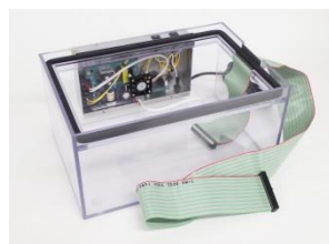
Test chamber for gas sensor evaluation (with signal cable)
