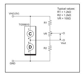
Fig. 2 - Basic measuring circuit
