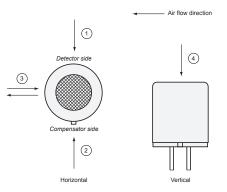
Fig. 15 - Air flow testing direction (ref. Table 1)
