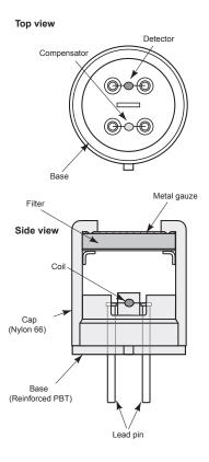
Fig. 1 - Sensor structure
